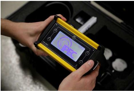
**PD-SG1** is used to detect, verify and locate PD activity in switchgear. The unit offers both TEV detection for internal discharge and ultrasonic detection for surface tracking and corona.
